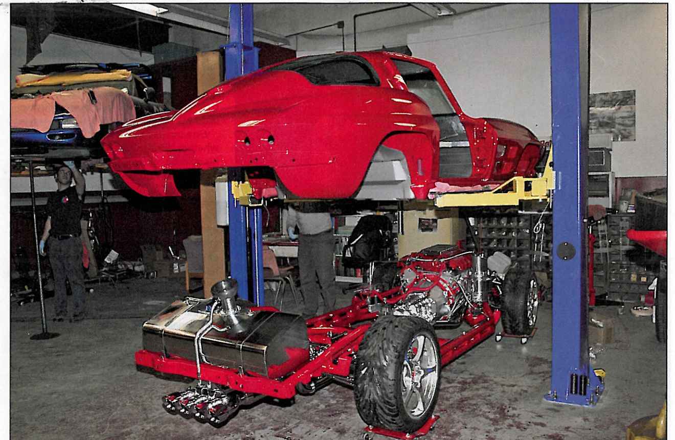
Getting ready for the body drop on Split Personality. Note the use of two "post" lift and custom mounts for supporting the body when lowering onto the chassis.
