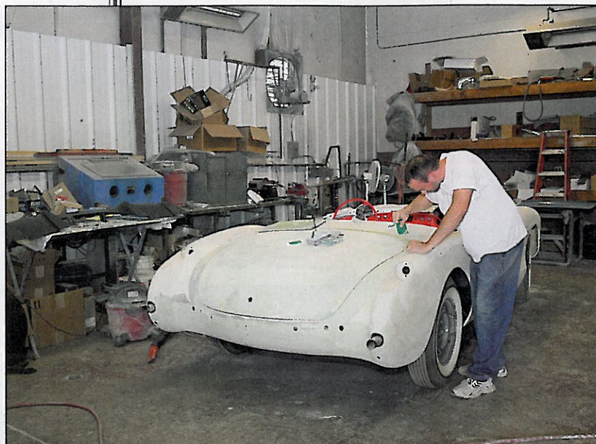
Preparation of a C1 body for painting in the body shop.
